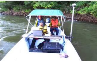
Odom - Dual Head Multibeam bathymetry mapping riverbed structures and morphologies of Tapajós River (Amazon) - MB1
