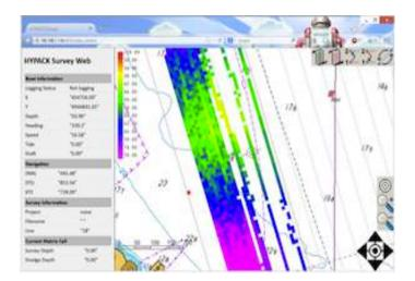
. **Single-beam editor -** Target Support: A Target dialog appears with the XYZ coordinates of your selected position and the default name (time) and target group (SBMAX).
